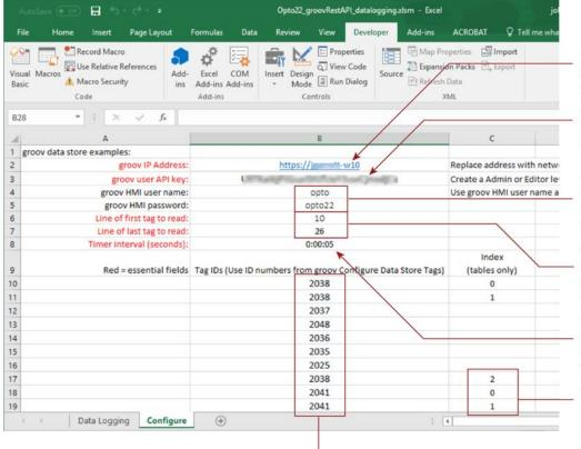
These are tag IDs from the sample *groov* project's data store. Change these to add or remove data fields from the data logging. Provide the IP address of the *groov* server or box that is running the *groov* project provided with this sample.
