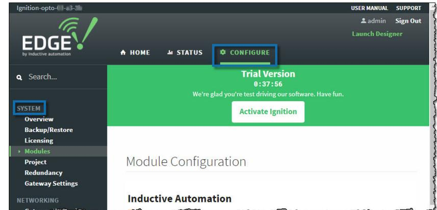
4. Scroll to the bottom to find MQTT Transmission, and then click its install button.
