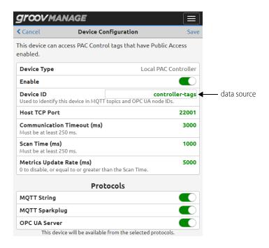
Notice the Protocols section. By default, all protocols (MQTT String, MQTT Sparkplug, and OPC UA Server) are enabled. You can disable the ones you're not using or leave them enabled for the future.
