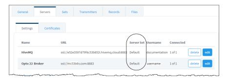
Ignition Edge allows you to create additional failover groups under the MQTT Transmission > Settings > Sets tab.
