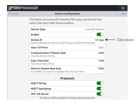
groov Manage will generate a topic path based on the ID fields in combination with others required by Sparkplug B. Subscribers can use a path with a specific tag, or use a wildcard (#) to subscribe to all public tags at that point on the path:
