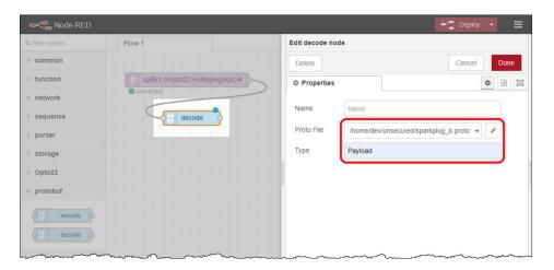
**6.** Connect the output of the Decode node to wherever you want to send the subscribed data, and click Deploy to start receiving data.
