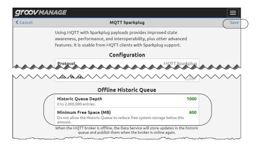
Note that records are stored to disk and will be lost in the event of a power cycle or power failure.
