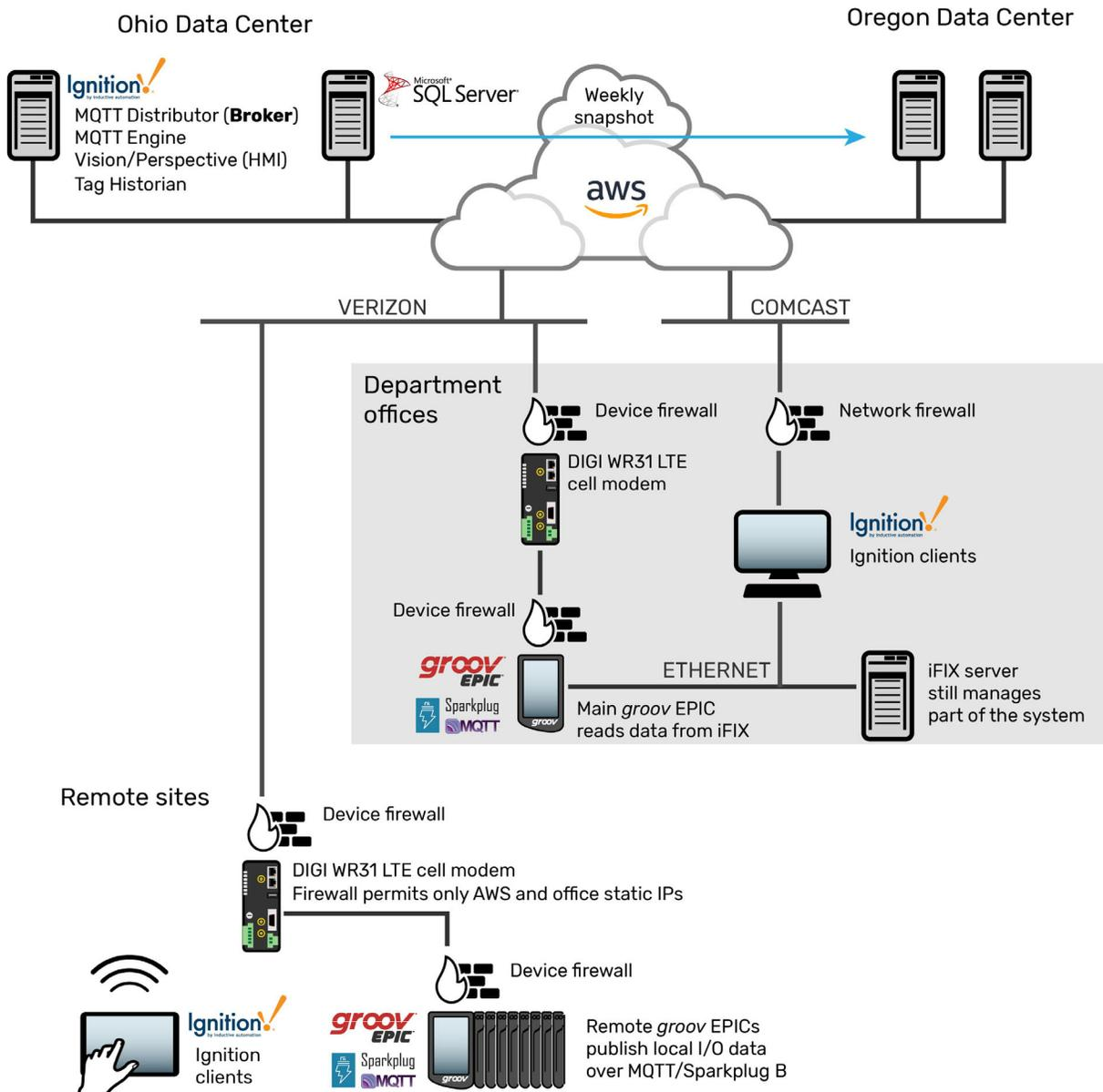
**Waterford DPW's modernized infrastructure publishes data from groov EPIC controllers to a cloud-hosted Ignition SCADA and MQTT broker over a 4G LTE cellular network.**
