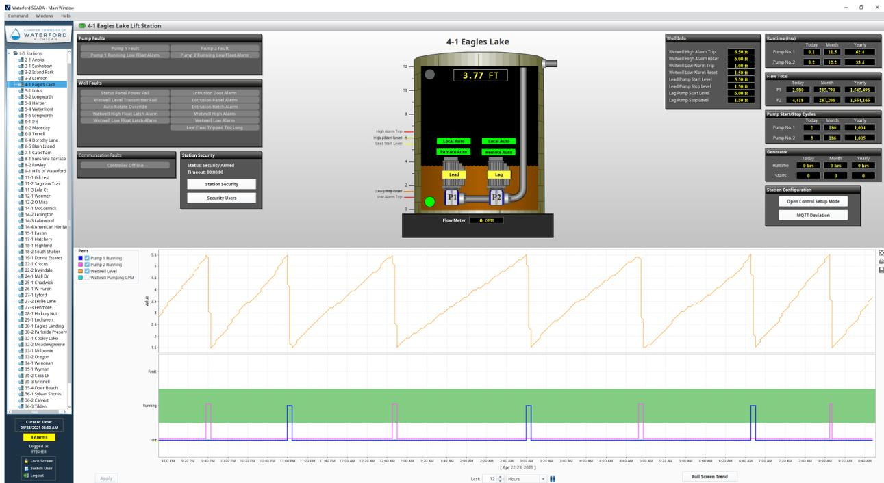
One of Waterford's new lift station control screens. The station security panel is shown at center left.
