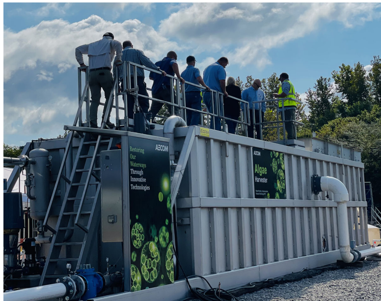
Observers watch the land-based 1 MGD harvester operating at the award-winning project site at Harsha Lake in Ohio, September 2022.
