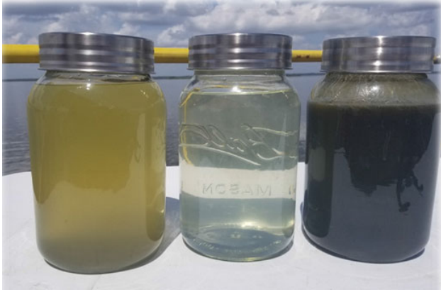
From left to right: raw lake water, HFT-clarified water, and recovered algae biomass
