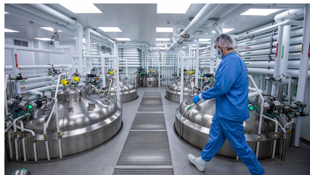
Fill and Finish Tanks in production
