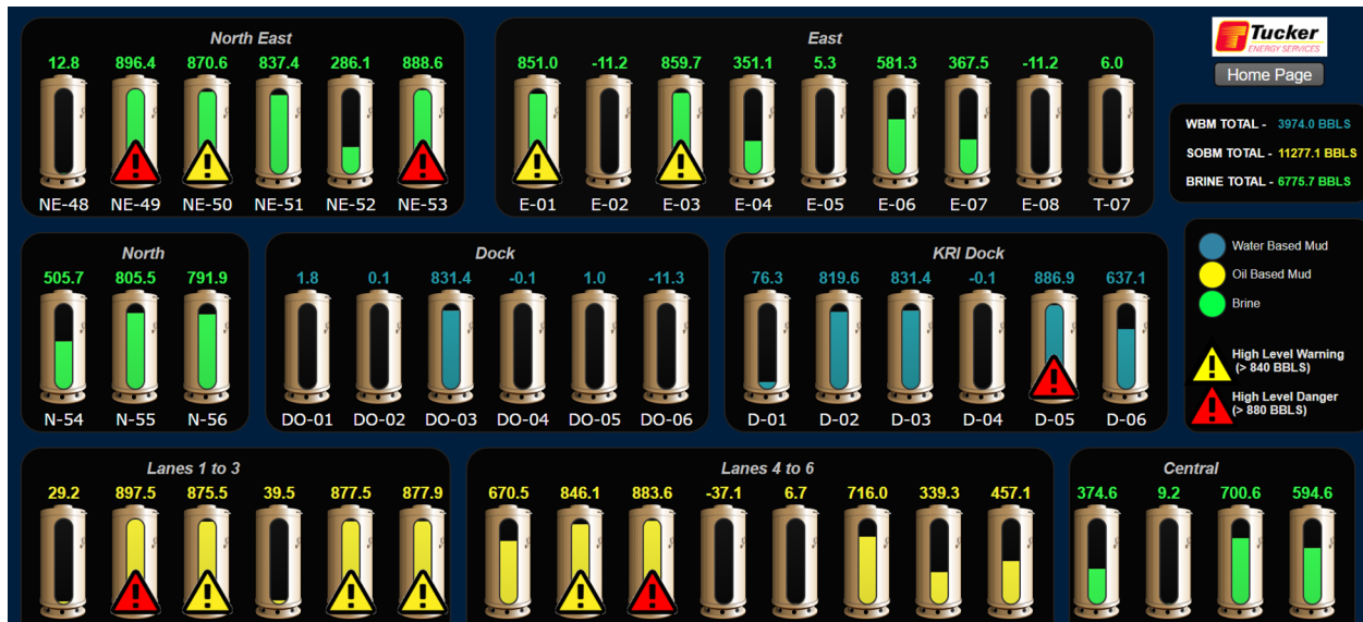
groov View tank monitoring screen
