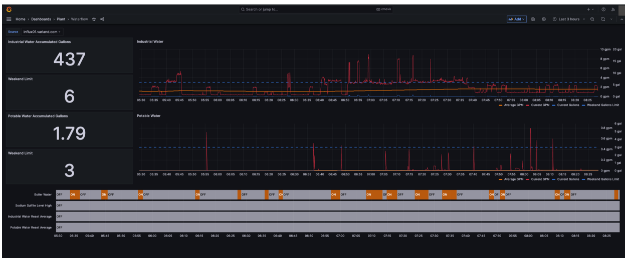
Varland Plating’s waterflow data visualized in Grafana via Opto 22’s REST API
