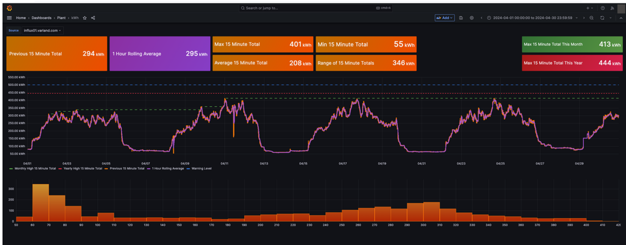
Varland Plating's plant kilowatt-hour data visualized in Grafana via Opto 22's REST API
