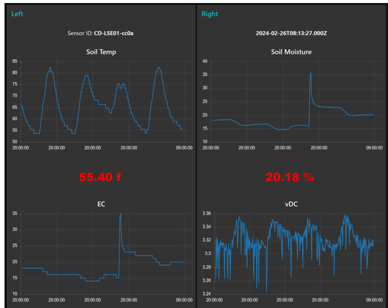
A dashboard displays soil temperature, electrical conductivity, and volumetric water content.
