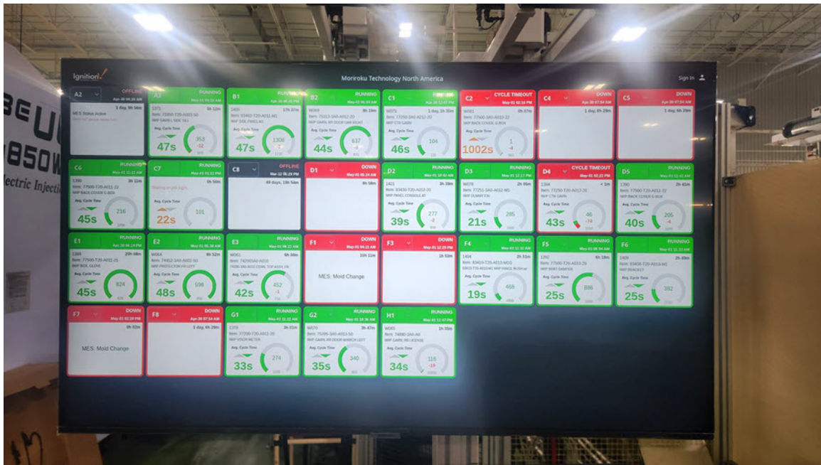
MTNA monitors a production dashboard built in Ignition.
