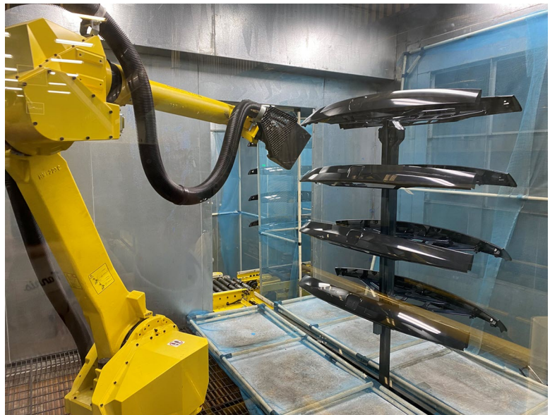
Robotic painting process for automotive exterior components
