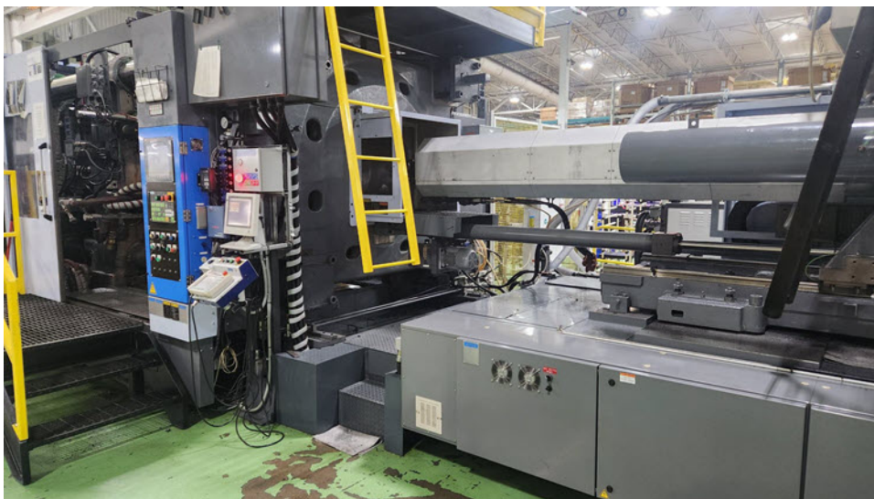
MTNA machines are used for high-volume injection molding.
